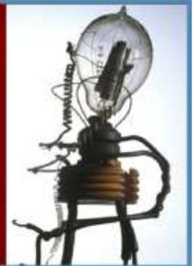
effective, they needed significant power, space to keep from over-heating, a steady flow of replacement vacuum tubes, and were too bulky to fit in smaller applications.
